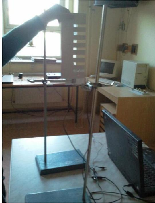
Figure 2: Free fall of a paper comb
