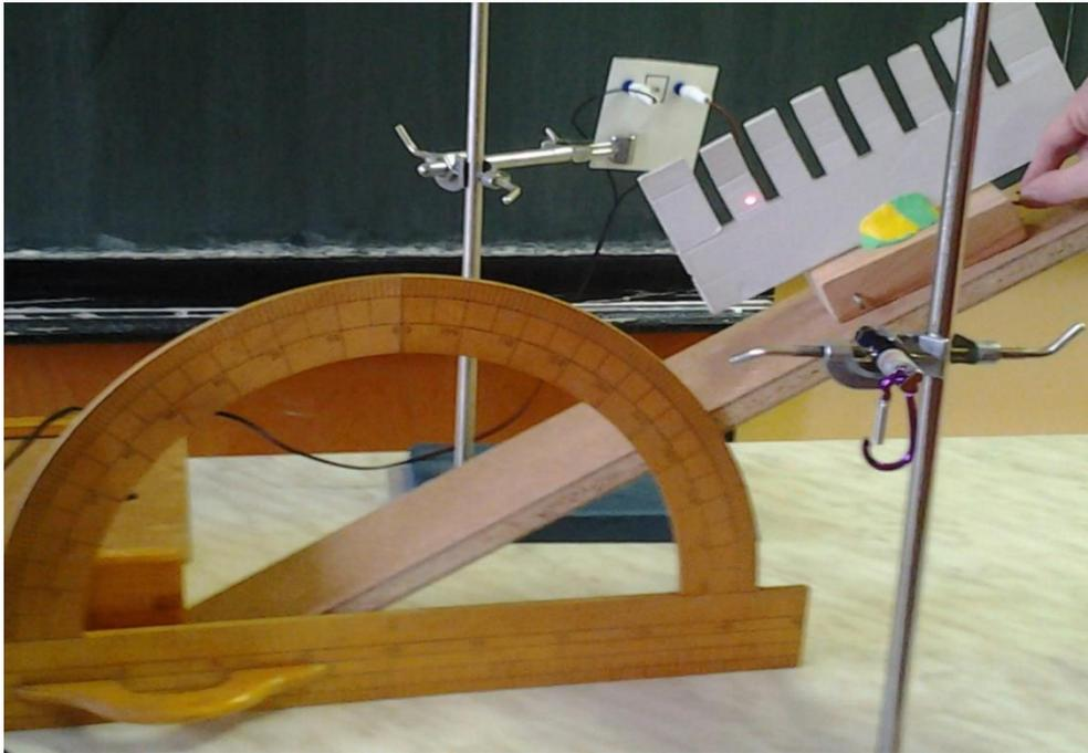
Figure 5: Measuring of the coefficient of the friction
