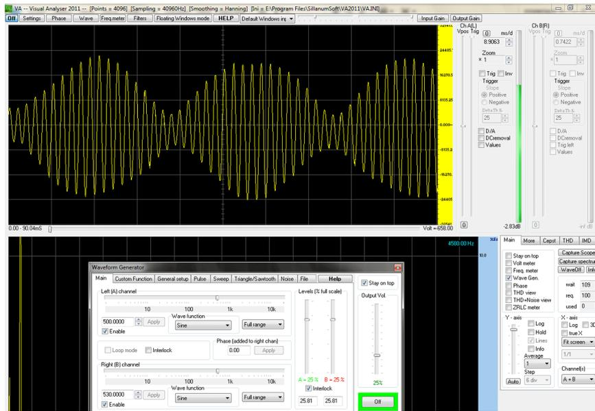
Figure 6: Sound beats by using the Visual Analyser
