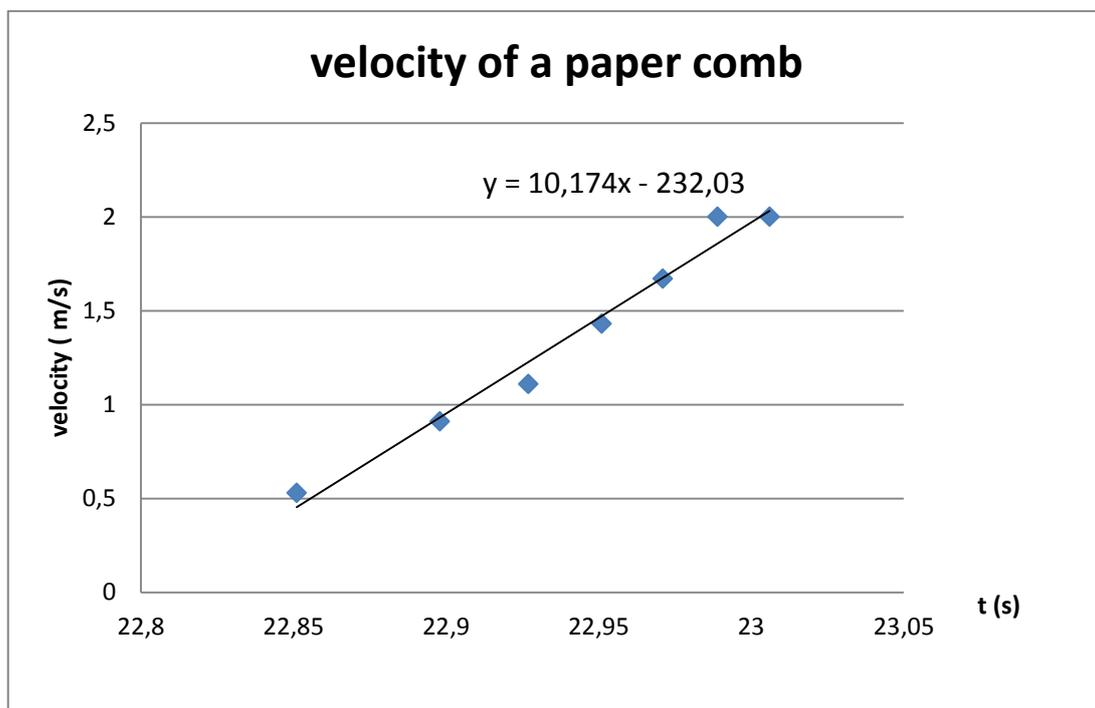
Figure 4: Free fall of a paper comb – MS Excel graph with linear regression
